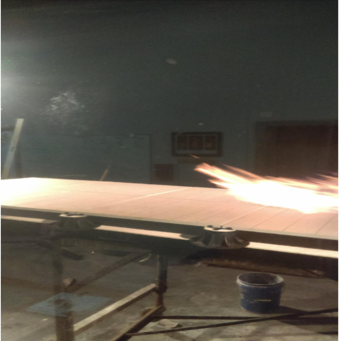
**Photograph 5 Parallel, Porcelain pavers at Maximum Flame Spread**
