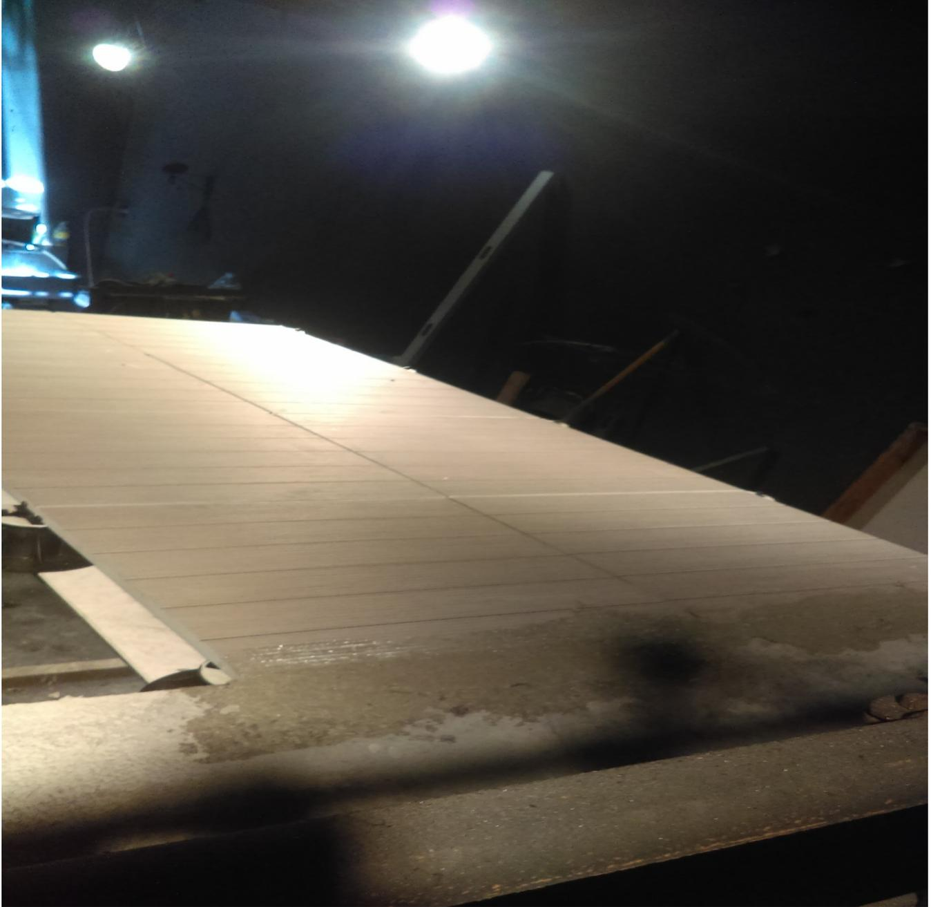
**Photograph 4: Parallel Porcelain pavers Prior to Testing**
