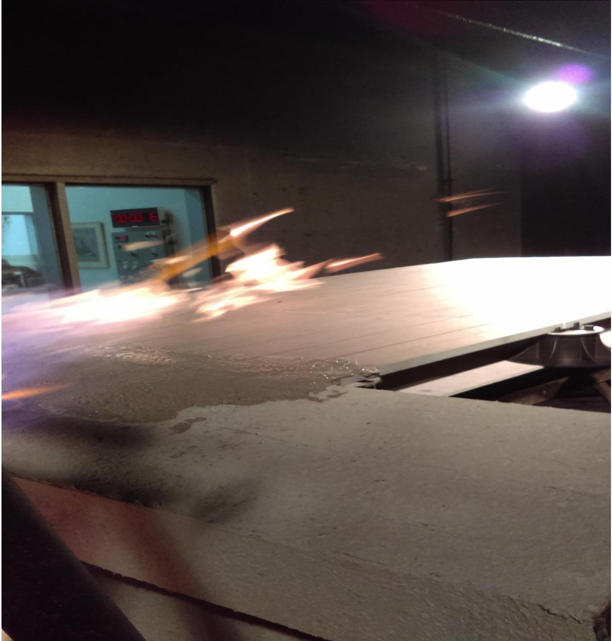
**Photograph 2 Perpendicular, Porcelain pavers at Maximum Flame Spread**
